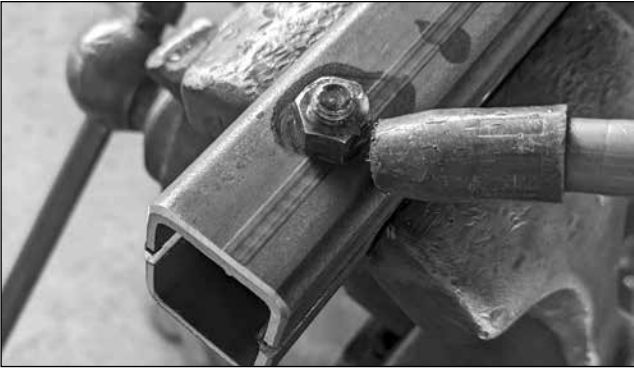
Fully weld the nut in place. It may take a minute before you can un-thread the bolt
