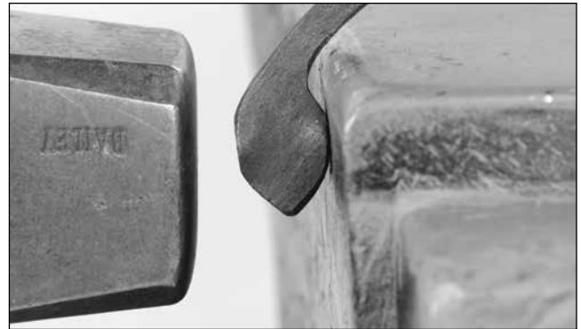
Leave room under the taper as the bar will move closer to the anvil
