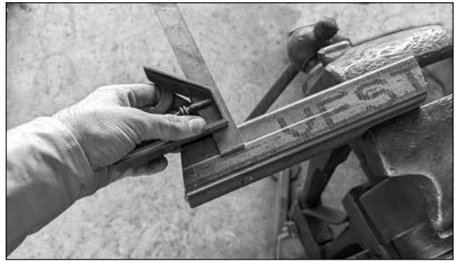
Use a square or dividers to mark a central line along both sides of the outside legs
