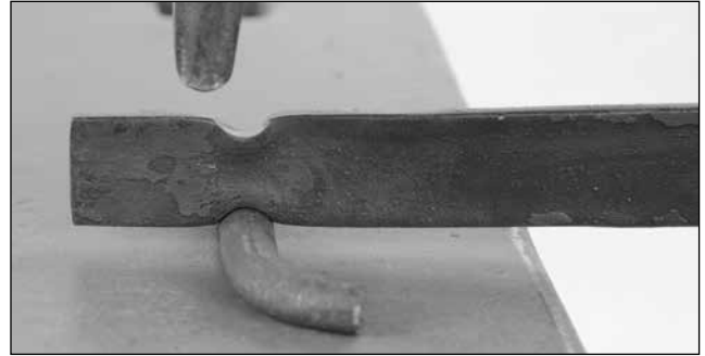
Never fuller to the full depth that you require. Hammering will also add to the fullered depth
