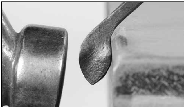
And then lower the barstock to remove the other corner. You should be left with a lemon shape
