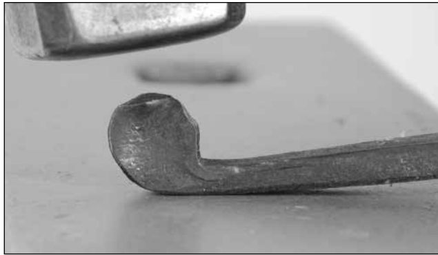
Drive in the remaining corner rocking the bar back and forth as you do so, preventing a flat spot on the back
