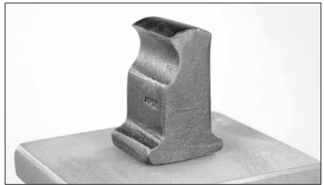
A tool that can be used to dress the finial. This tool is optional and not required for a great ha'penny scroll
