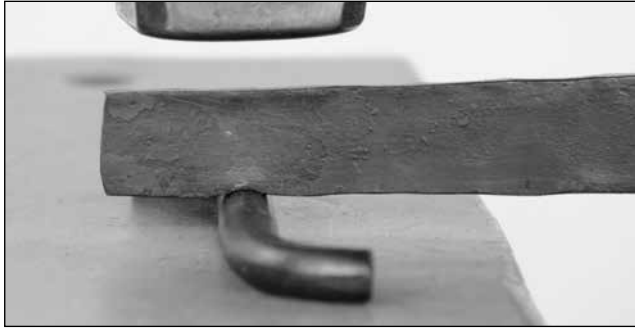
To start, create a shallow divot on one side of the bar
