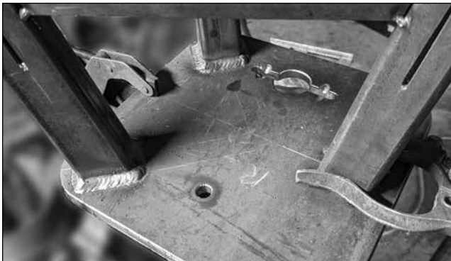
Once everything has been tacked in place, fully weld all seams. Distribute the heat as much as possible
