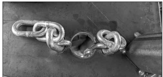
The bottom of the plate showing a method of retaining the ends of the chain. Chain fitted shown below
