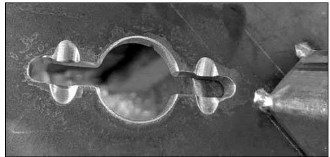
The bottom of the plate showing a method of retaining the ends of the chain. Chain fitted shown below
