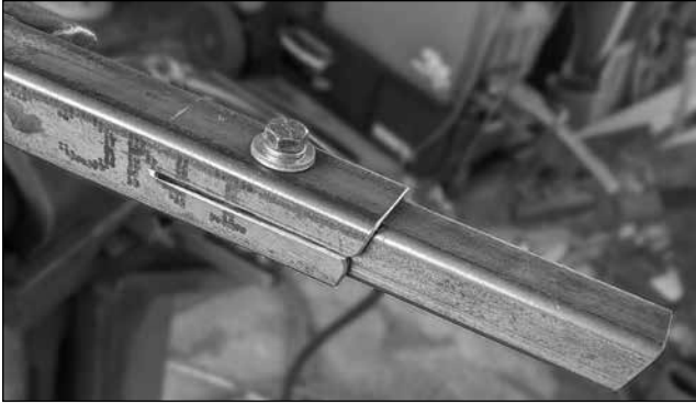
Here is a view both legs fitted together showing how the adjustment works
