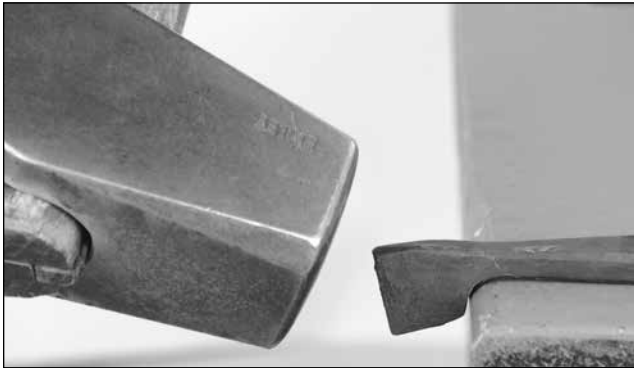
Using a glancing blow, knock in the top corner of the flag
