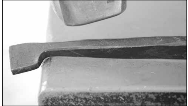
Chamfer at least the edges of the taper. I like to chamfer the whole bar as it aids in fitting the collars
