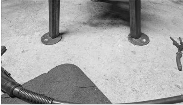
Round, pre-drilled plate make the feet for the stand
