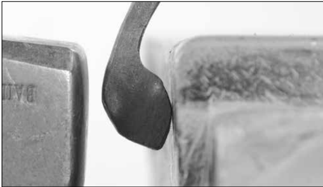
After creating the flats, knock off first one pair of corners by raising the barstock...
