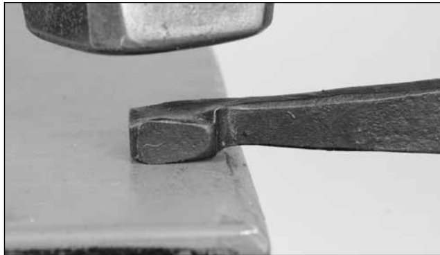
Work near the offside edge to prevent damage to the taper as you dress the now-square flag
