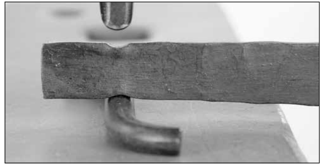
Having the divots in place really helps reduce the balancing act, and aids accuracy when combining the tools
