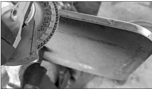
Dress the edges of the cut. Make the edge safe for you or your co-worker
