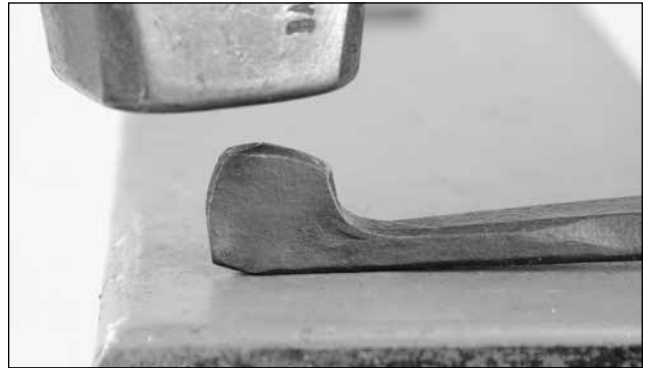
Flatten the top surface until it is parallel with the surface of the anvil
