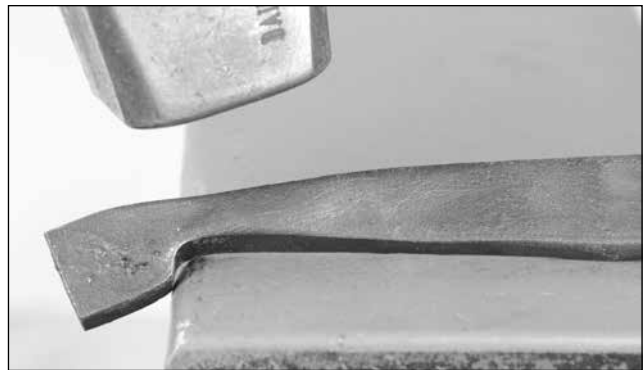
Turn the bar 45°, and work from the top and sides only so as not to damage the 'flag' of material
