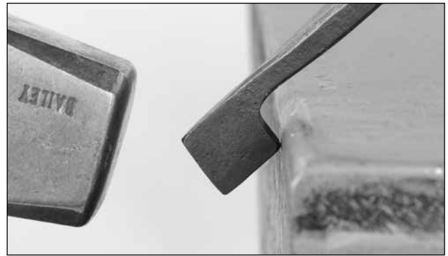
Hold the bar at a 45° angle to the anvil and drive in the outside corner.
