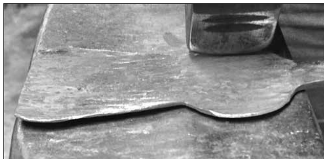
Now work the circle. Keep your hammer parallel to the centerline throughout the spreading sequence unless things go wrong
