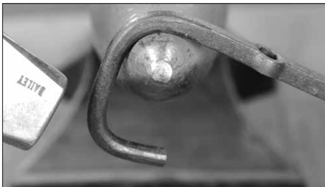
Taking the bend past 90° can make it easier to catch the bick when you turn the link over
