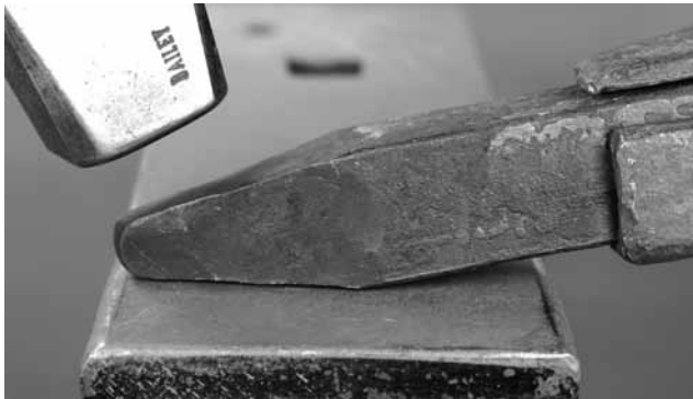
Dress the taper on the face of the anvil
