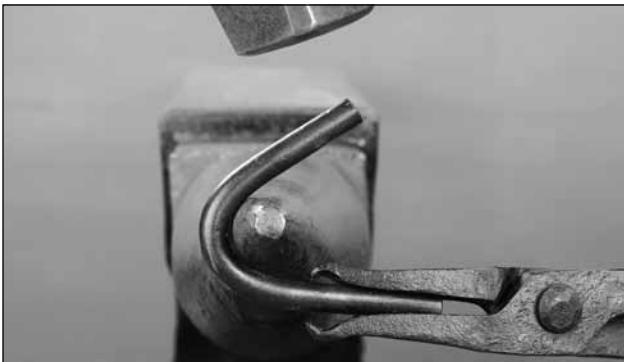
Keep an eye on the length of the arms, try to keep them of equal length. Stop if they get out-of-whack.
