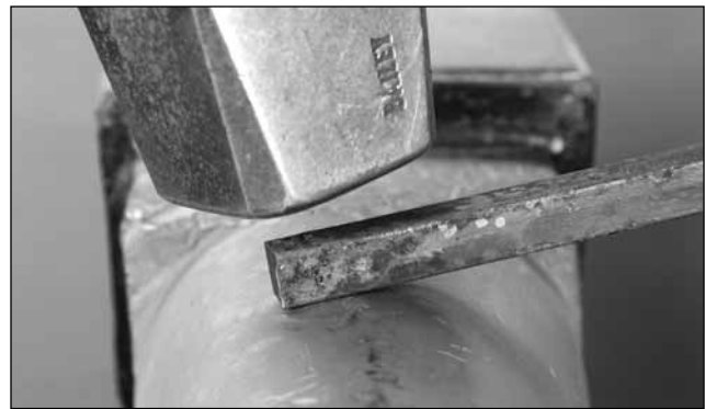
Draw down a length of \frac{3}{8} -inch square bar on the bick
