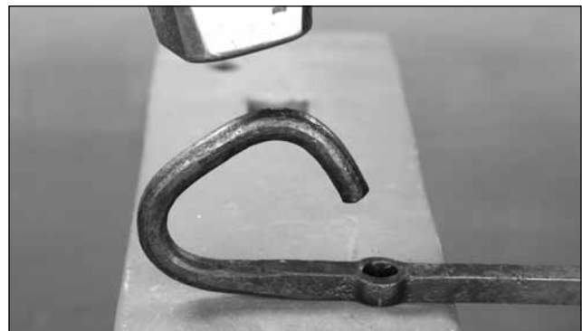
Close the link on the face of the anvil and give it a good brushing before returning to the fire
