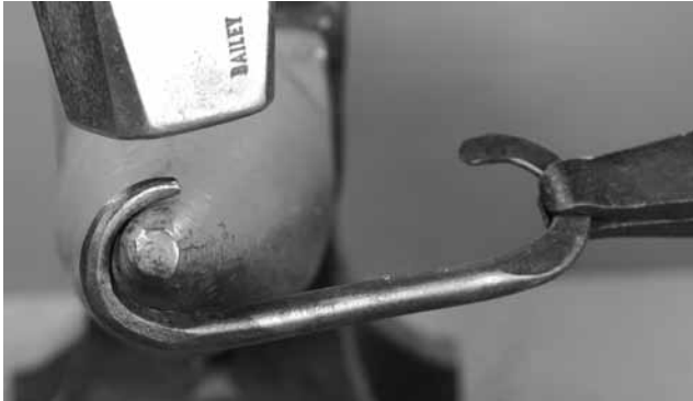
Leave the end slightly open of 180°
