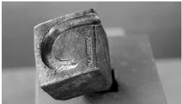
The swage is fit close to the positive form to allow angled hammer blows during use
