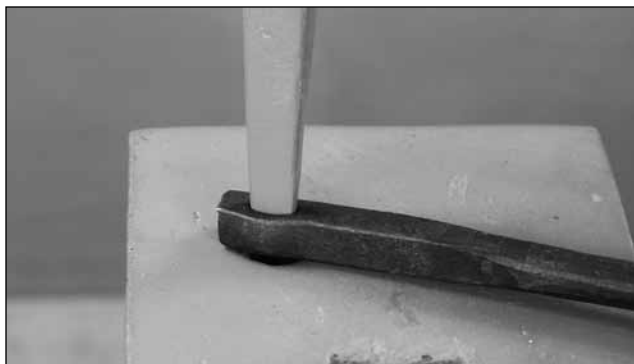
Clear the slug over the pritchel hole
