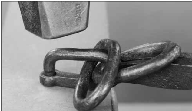
Here the repair link applied to two links of chain
