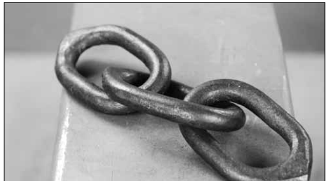
For longer chain, create several 3-link lengths and the use a 7 th link to join 2 lengths together
