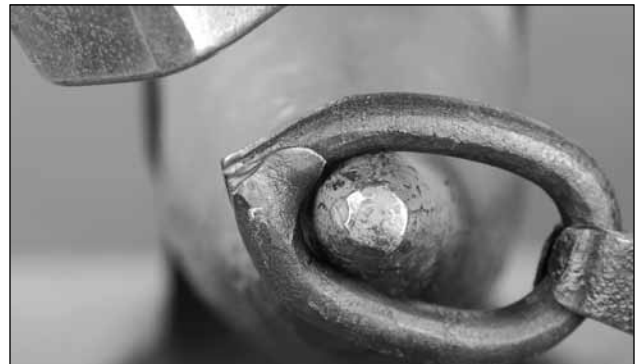
You might need to level the ends so that the points are aligned
