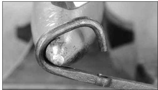
This is a far as I go on the bick before moving to the face of the anvil
