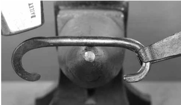
Turn the link over a 1-inch part of the bick
