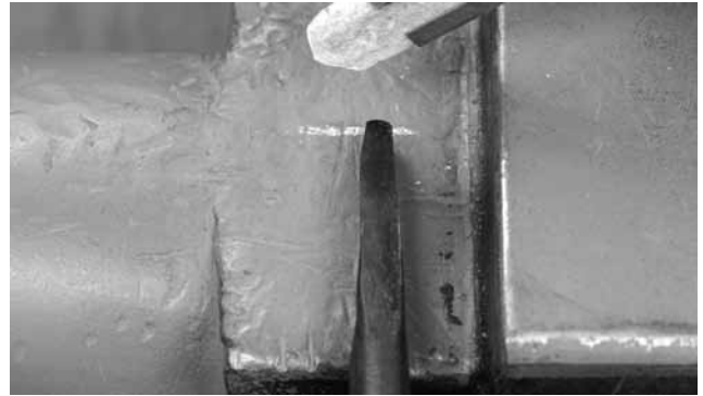
Record the actual length of taper on the step to aid in making the 2 nd end equal
