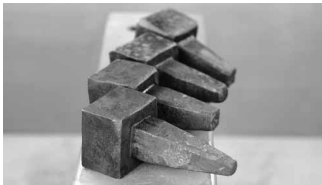
I use a gas forge and make bottom tool blanks in sets of four
