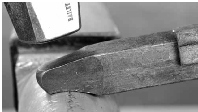
Draw down the first ⅓ of the bar into a blunt taper over the bick
