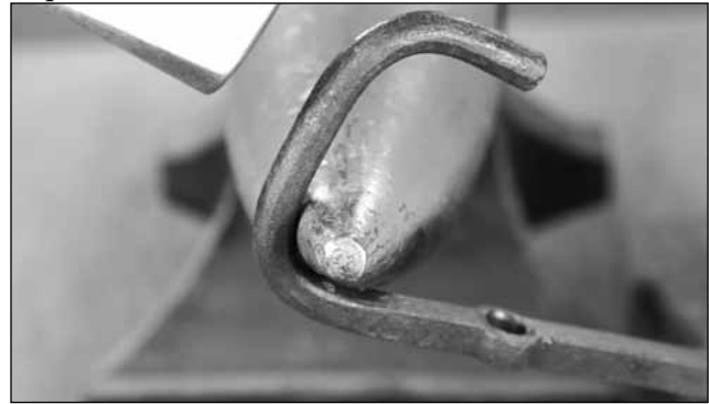
Finish the bend over an appropriate part of the bick, leaving an ID that matches the chain link
