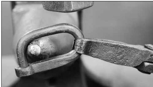
Open the repair link at the bick or with tongs, ready to apply the two ends of the broken chain
