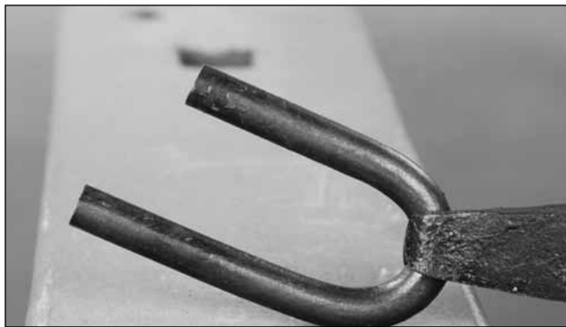
This isn't good either. Change the shape from a U to an open V and tap the high side down
