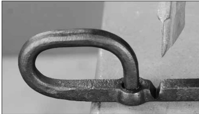
Sever the repair link from the parent bar and hot rasp the cut end either flat or curved
