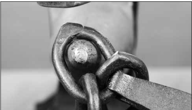
I try to keep one link either side of the tong jaws as I continue to weld on the bick
