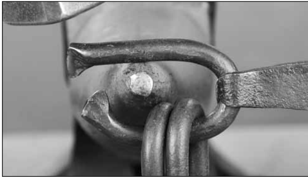
Turn the second end in and close the gap. Note that the welded links are beneath the tong jaws.
