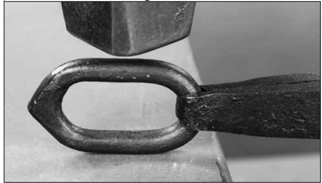
If your link is a little wonky, dress it on the face of the anvil
