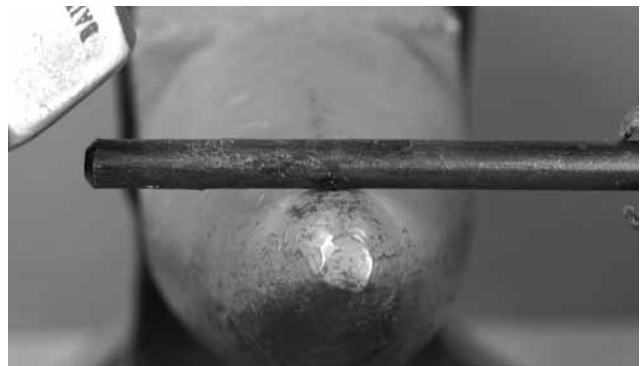
Turn the end over a 1-inch diameter section of the bick
