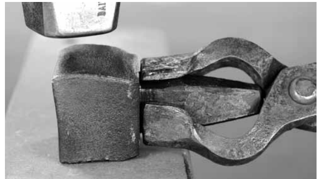
A final dressing of the sides and then top of the bottom swage
