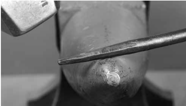
Turn the taper around the bick
