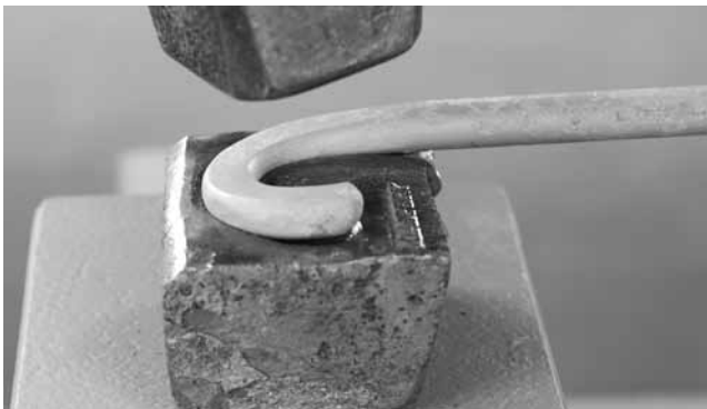
The depression should be the deepest on the straight-away and shallowest on the free end
