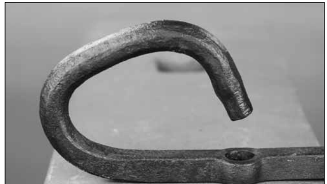
A variation is to create an appropriately sized hammer-forged tenon on the end of an oversized round section
