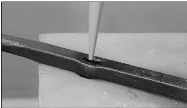
I use a tapered drift when drifting the mortise, but that's personal preference
