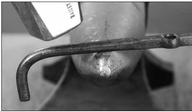
With an allowance for the material needed to make the bend, turn the repair link
