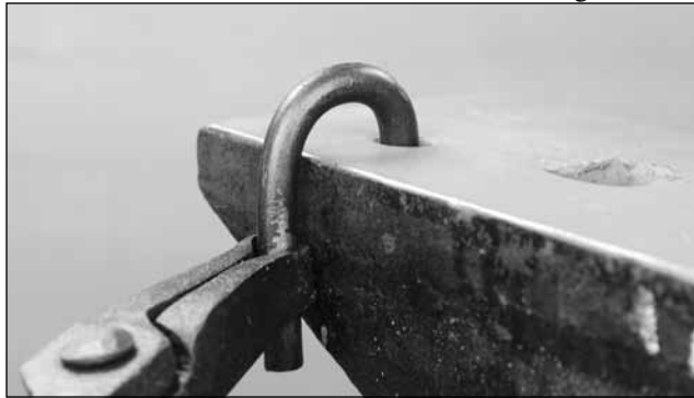
Use the vise or the pritchel hole to take out the twist
