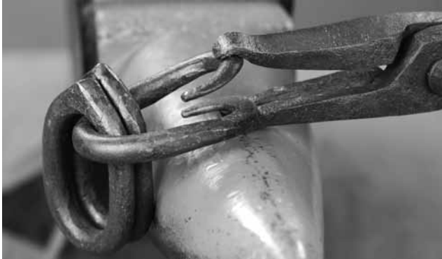
The split link being applied to two chain links for display on my project board
