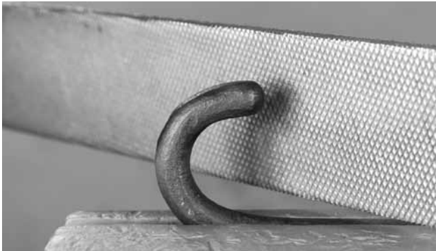
Hold the part horizontally in the vise as you hot-rasp the end to a half sphere shape. Quench on completion.
