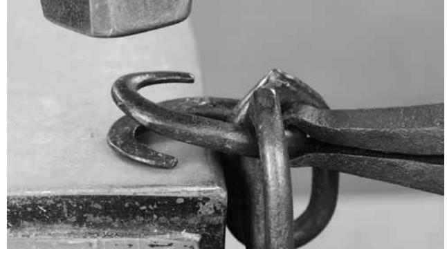
Set the gap to prevent losing the two chain links then brush and wax for display
