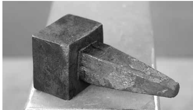
This is the blank that you are aiming for 1⅜" plus tall and about 1⅞" to 2" square on the face
