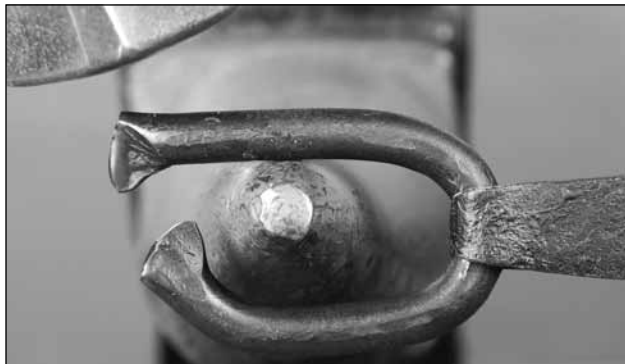
Bend the second arm around the bick
