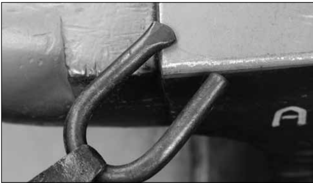
Keep hammering and pivoting to create the slope of the scarf
