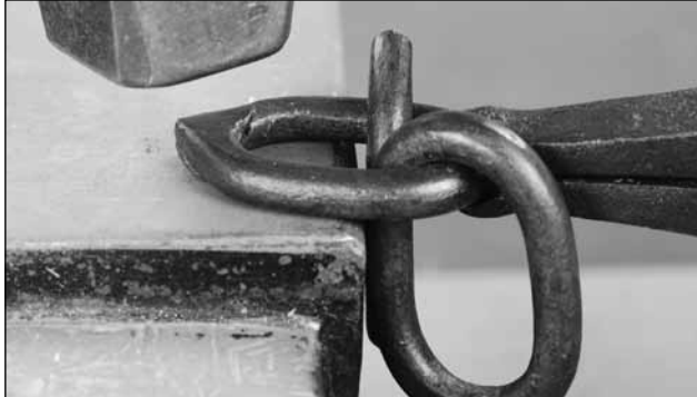
The trick now is to weld without letting the other two links get the better of you in the process
