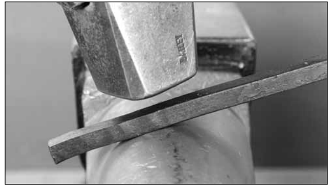
Draw down a 4-inch length to a \frac{5}{16} -inch square cross section
