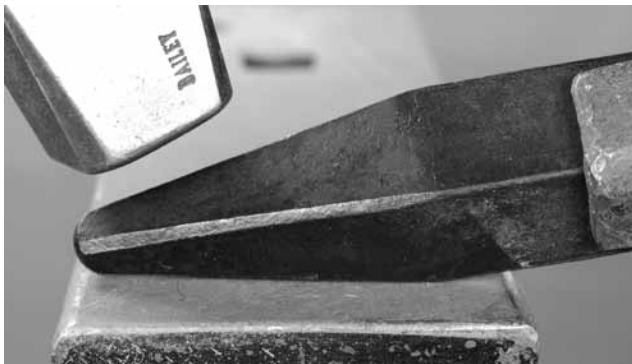
Chamfer the corners in preparation to resist fire damage as you take the high heat needed for upsetting the bar
