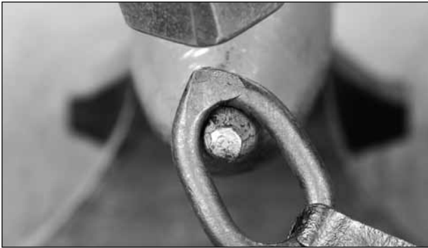
Have the apex tilting towards the heel of the anvil as you work
