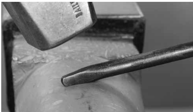
Draw a 1¾-inch long square taper to the end of the bar
