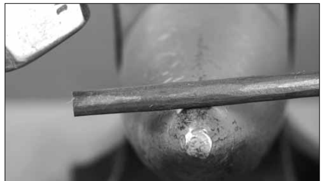
Lay off about 1 \frac{3}{8} -inch from the center of the bick
