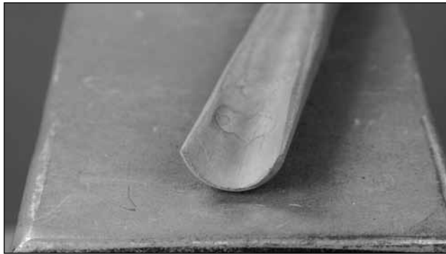
A curved chisel can prevent 'rabbits ears' on the end of the bar post drifting
