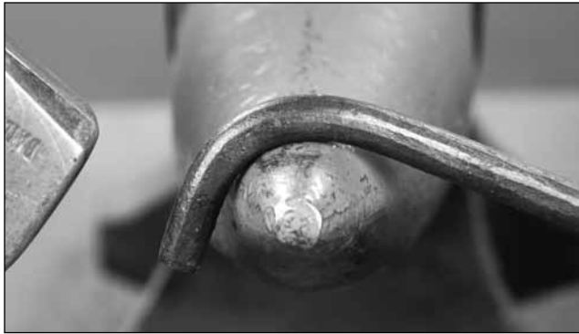
Bending the bar to slightly past 90° makes it easier to thread the tenon into the mortise
