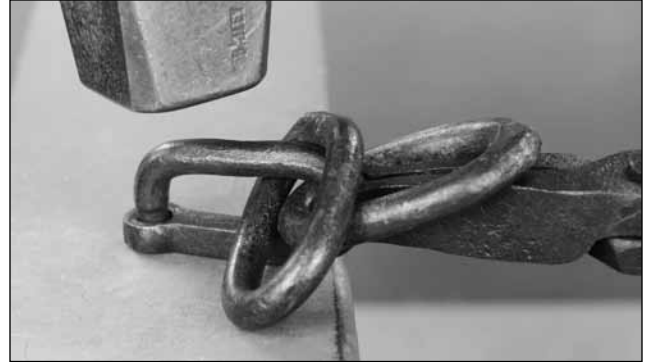
Here I've added two links of chain to show the application of the repair link
