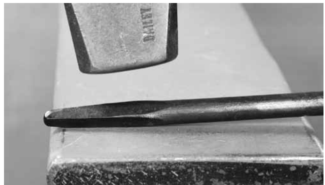
Dress the taper and take to an octagon cross section
