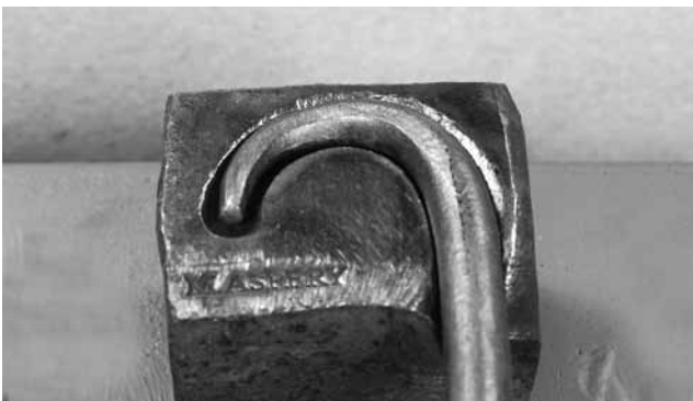
The taper should run along the centerline of the depression - and fit not quite to the end
