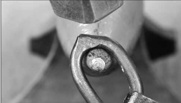
Weld the upper and lower seams at the same time
