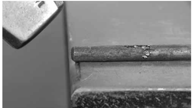
Quickly chamfer one end of a 6-inch bar and go to the bick
