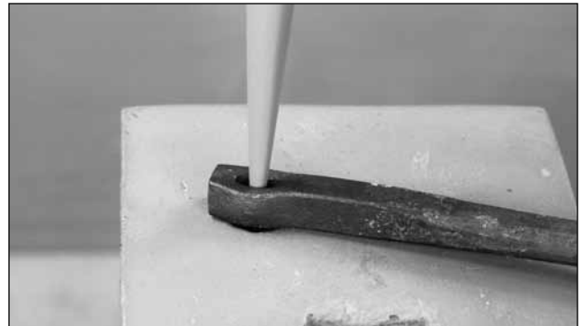
Using a tapered drift, open the hole working from both sides of the bar as you go
