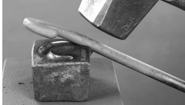
Knock off any sharp edges from the swage
