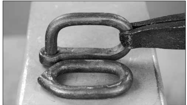
The repair link should be of a similar size to the chain being repaired
